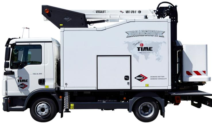
Top of the line access platforms mounted on larger vehicles capable of providing the best possible elevated work environment. Booms are fabricated from high strength steel providing the most stable and safe cage experience available on the market.
